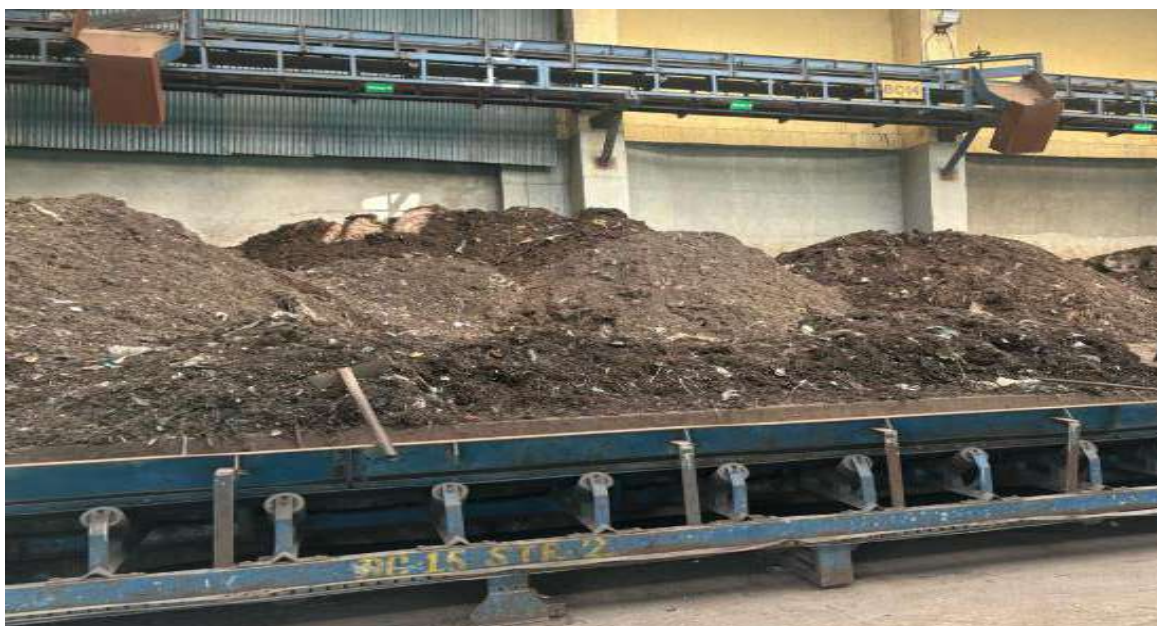
Figure 11 C: Enclosed area for composting
