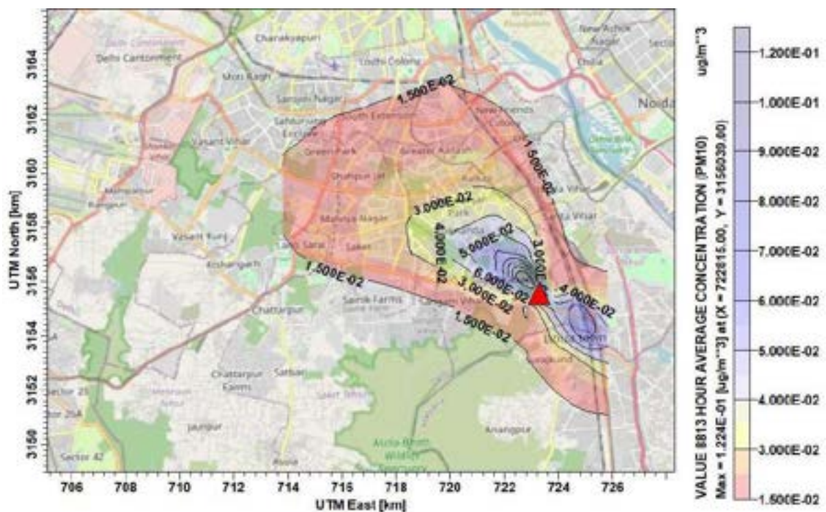
Figure 30: Isoleth of annual average GLC of PM around Ghazipur WtE plant.
