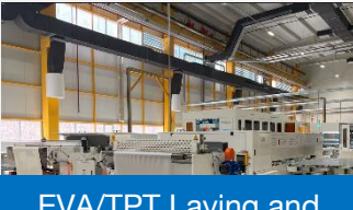
EVA/TPT Laying and Cutting machine
