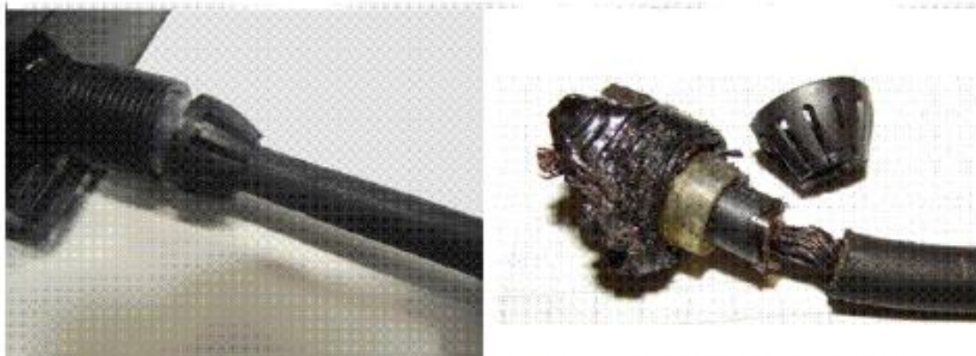
The faulty examples for rework cable of junction box.
