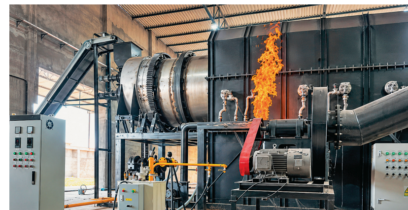
Beyond Drilling & Exploration Pvt Ltd Kaljharani Bhatinda Continious Torrefied Biomass Plant producing 200 tons per day
