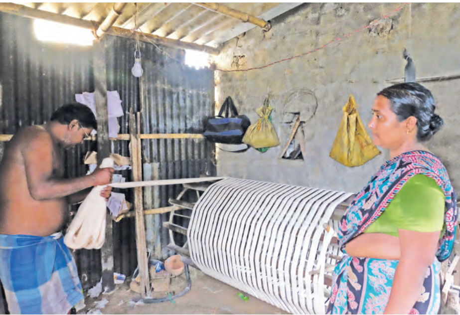
Yarn is cleaned, strengthened, dried and straightened on drum-like wooden structures
