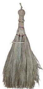
Gajra jhadu is made of date-palm leaves and is used to sweep cement surfaces
