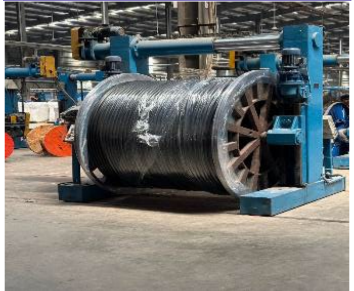
Exhibit 22: Final outer layer processed
