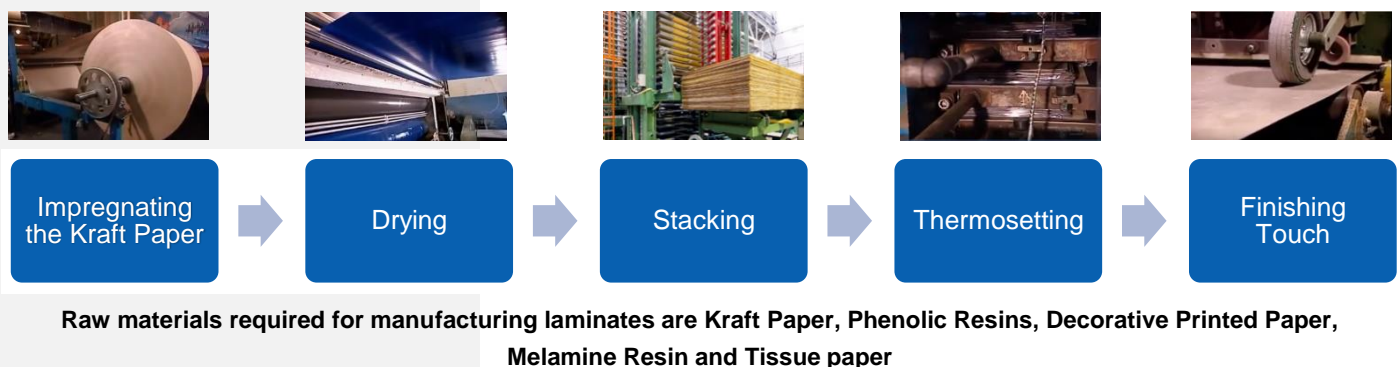
Exhibit 41: Manufacturing process of Laminate Sheets
