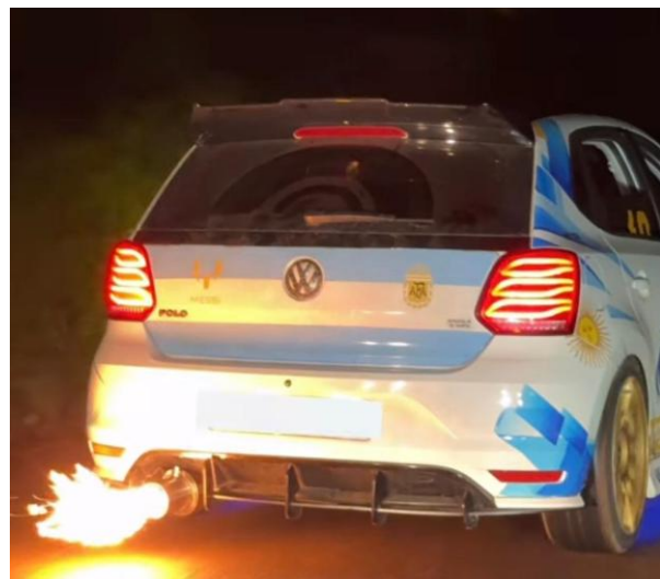
(Flame emitting from after-market exhaust systems with 'flame-kit' fitted on a diesel car)
